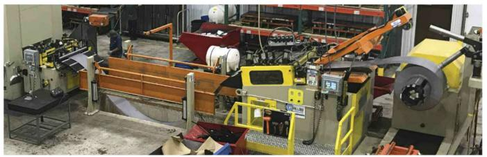
Along with its new mechanical presses, Manitowoc Tool & Manufacturing has invested in the latest coil-handling technology to feed them. This 48-in.-wide-capacity coil line feeds a Seyi 660-ton press, and gives the metalformer tighter control of material straight through the tooling while keeping the material finish pristine, a must given that Manitowoc produces a large amount of cosmetic parts.
